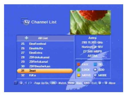
Press the OK button to access the channel list.
